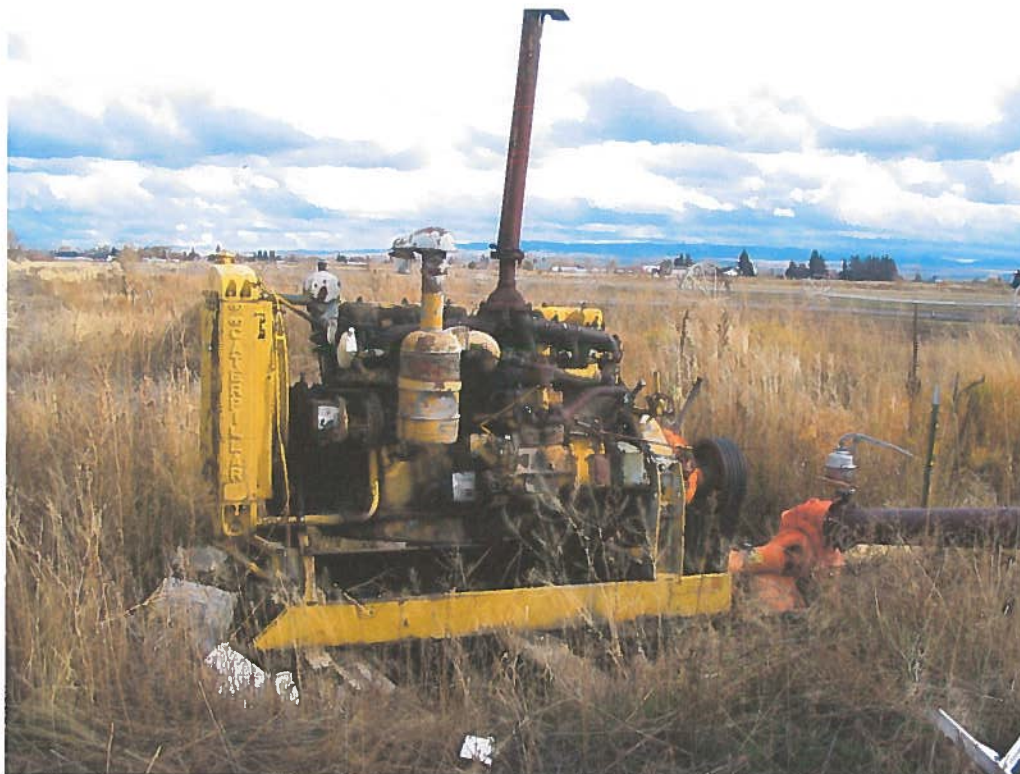
Rediversion pump on ditch, A22-631 + A22-636A
