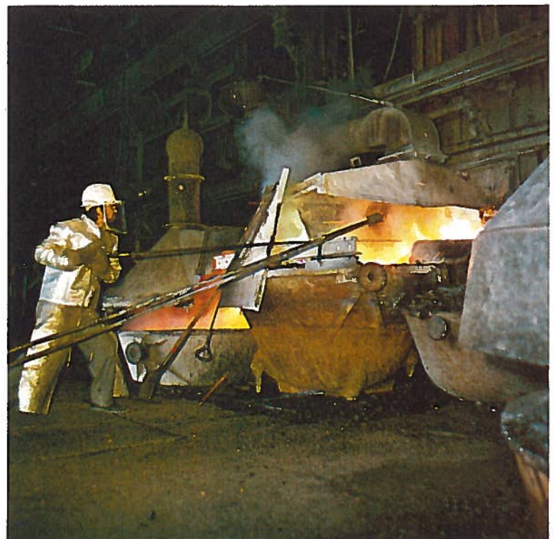
Below: Operator taps the Smelter blast furnace to permit molten slag to flow from the furnace.
