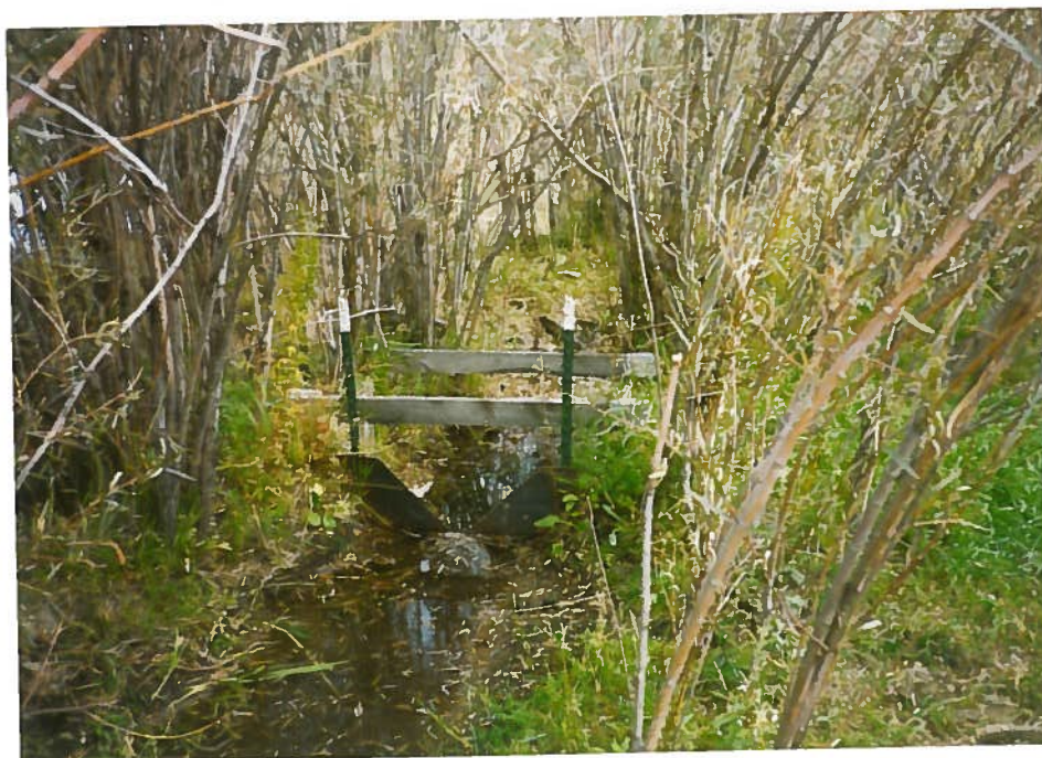
Curtis measuring device - 90° V-Notch Weir View Looking South.
