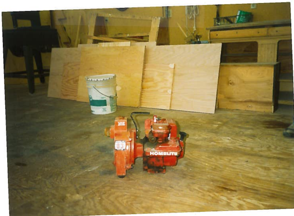
Small portable gasoline pump used by Bloxham, to lift water from stream channels for gravity irrigation of his pasture and garden areas.
