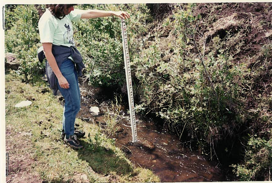
PHOTO #4 UPSTREAM MANNINGS CROSS SECTION. NOTE! DITCH WAS ONLY FLOWING ABOUT 2/3'S FULL.
