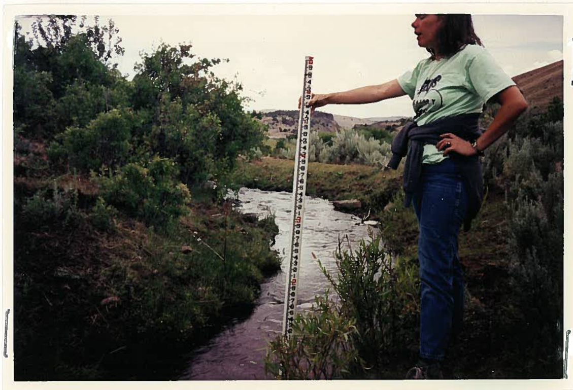
PHOTO #4 UPSTREAM MANNINGS CROSS SECTION. NOTE! DITCH WAS ONLY FLOWING ABOUT 2/3'S FULL.
