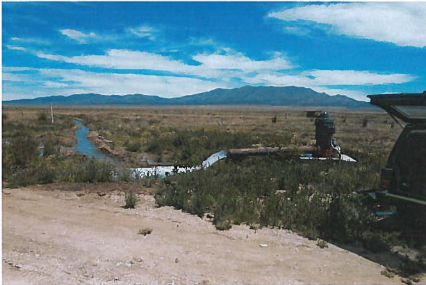
Figure 1: US Electric 125-hp motor. Serial number R2020949. GPS file name: T-62119A. Pump: Layne and Bowler, Serial number LP99061/12T. Flow was measured with the Polysonic flow meter at an average of 1573 gpm or 3.51 cfs. The ditch was a new dug ditch. There was some wild flooding going on at the top of the ditch because the ditch was not deep enough to handle to flow. The pump had been redone last year.
