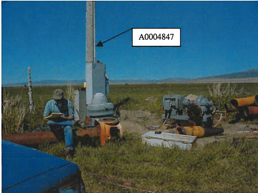
Figure 1 Denton Whitaker POD T14SR27E08 SWNWSE. Pump had to be reconditioned because of wear.
