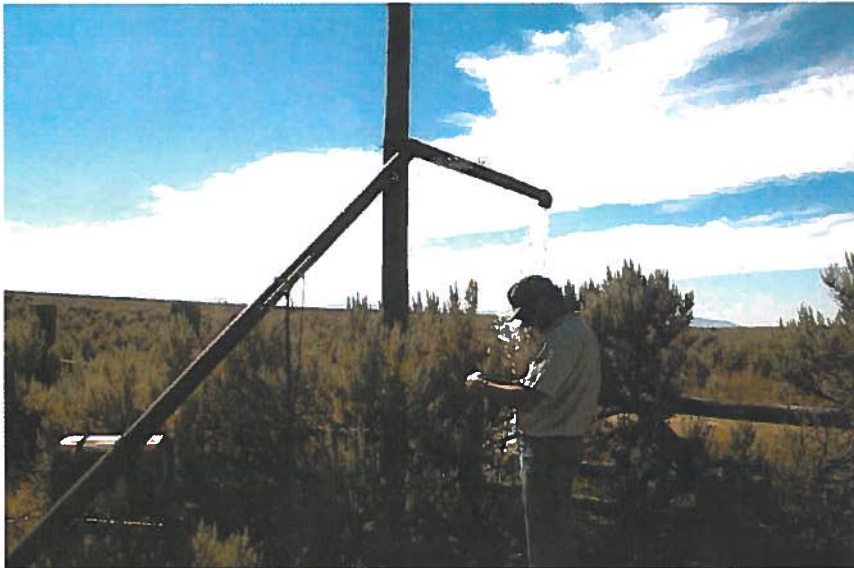
Figure 4. Scott King Data logging the flow for C Bar Cattle Company. Flow was measured at an average of 228 gpm or .51 cfs.
