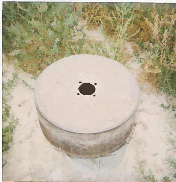
Tractor Belt Pulley used to develop wells with Panna Pump
