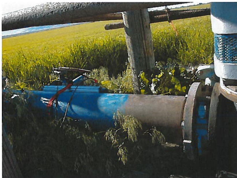
Figure 2. Fuji Flow meter transducer placement for Travis Whitaker. Average flow: 951 gpm or 2.12 cfs.
