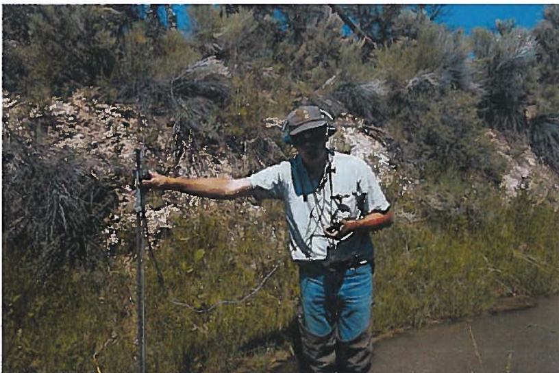
Figure 4. Scott King counting the revolutions using the Pygmy Meter. The flow calculation for the in stream flow was 3473 gpm.
