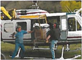
Crew loads a 800 # wood stove inside the helicopter. 91,000 lbs. of materials were delivered via 32 helicopter loads in 3 days. The route was 35 aerial miles to Big Creek from the main Salmon road.
