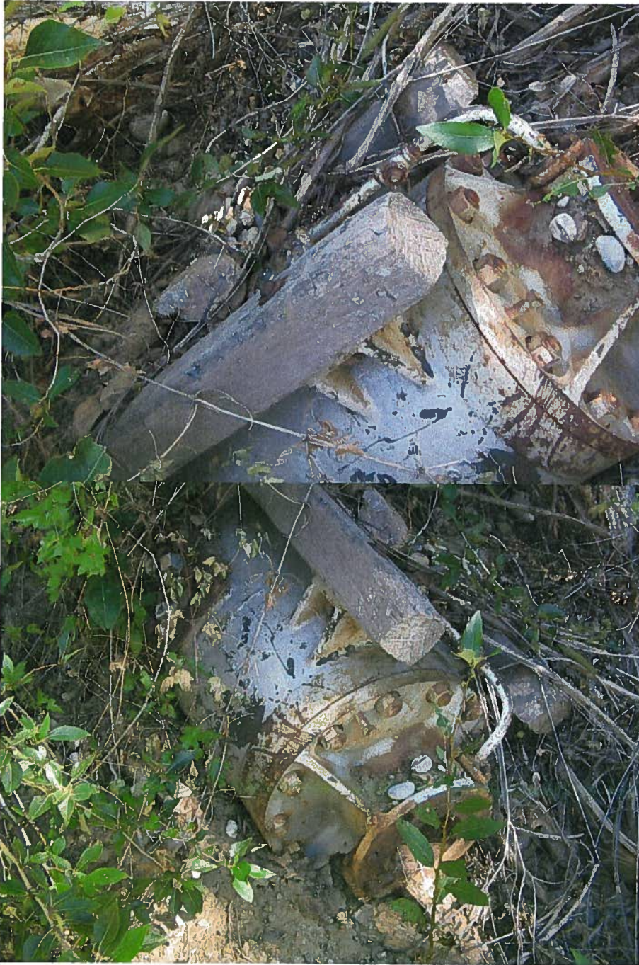
Photos of the old pump that used to sit in the Salmon River. At some point, Mr. Terry and another man tried to move the pump from the river to repair it. Mr. Terry tells me this is a 35hp pump. The pump has clearly not been used for a number of years, judging by the debris buildup around it and its general condition.
