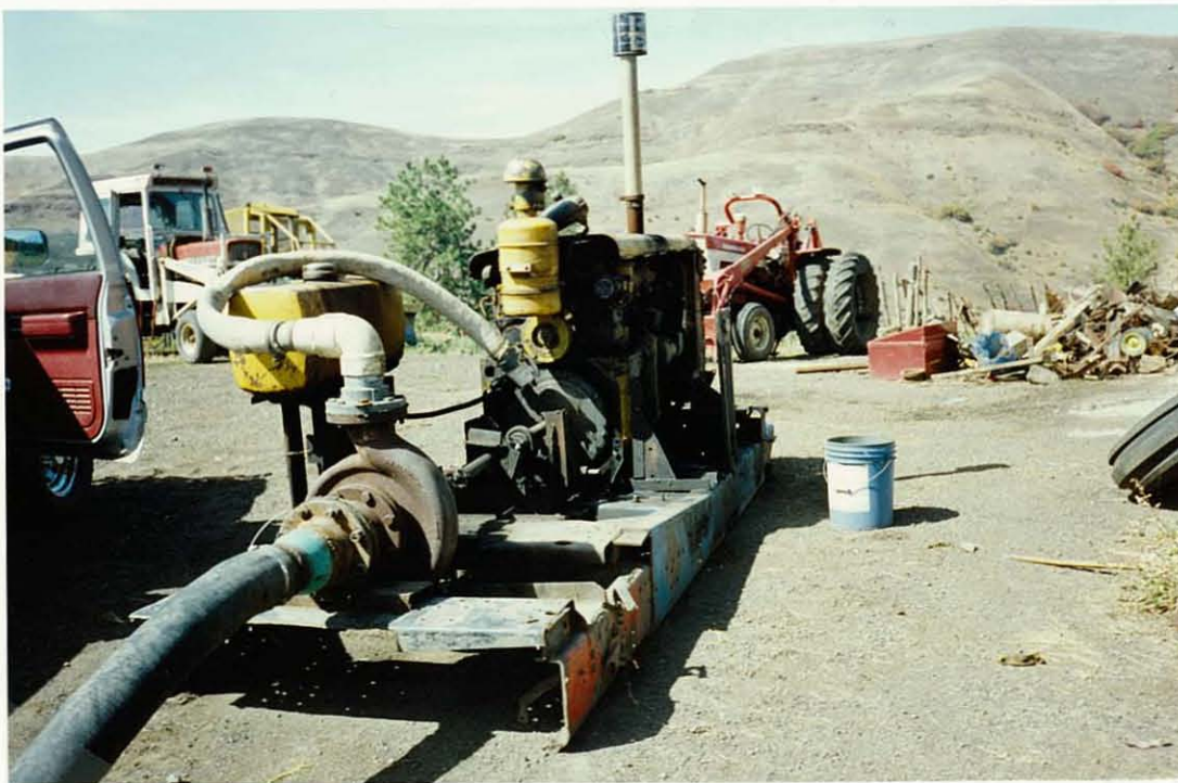
Portable PTO pump used to irrigate upper portions
