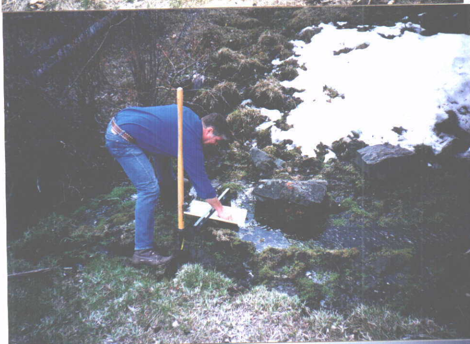
Photo 7. Al Ruberry MEASURING STREAM FLOW USING POWLUS V FURROW FLUME. MEASURED AT NWSENE SEC. 5.
