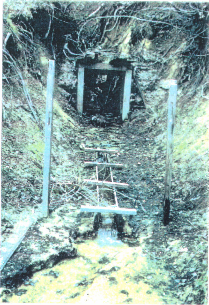
OVERFLOW PASSING THROUGH FLUME (eight inches wide) - Holidays, Fourth of July 1985 -
