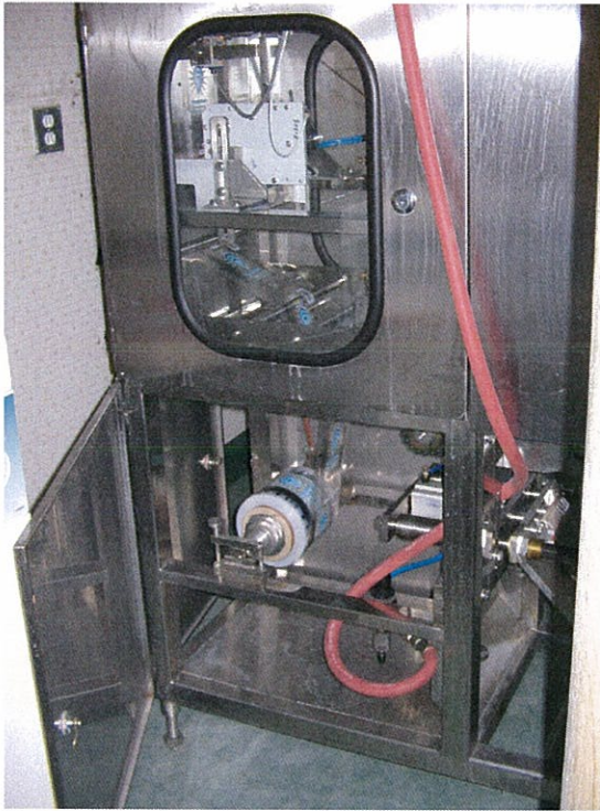
Part of the bottling apparatus. Technically, the plant does not use bottles, but plastic pouches. I use the term bottling here for convenience.
