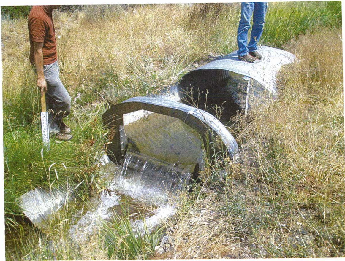
ABOVE: View of the measuring device (2.5 foot Cipolletti weir) on the Muldoon Ranch Company's middle diversion ditch. The head over the weir was measured at 0.42 feet, which would correspond to 2.29 cfs of flow. However, note that this device is located approximately 0.20 mile downstream of the Muldoon Ranch Company's middle diversion on Muldoon Creek.
