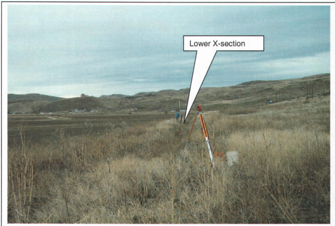
Photo 4: Lower X-section and level location of Manning measurement of the North Ditch. Located in E1/2 SENE, S31, T05N, R02E.
