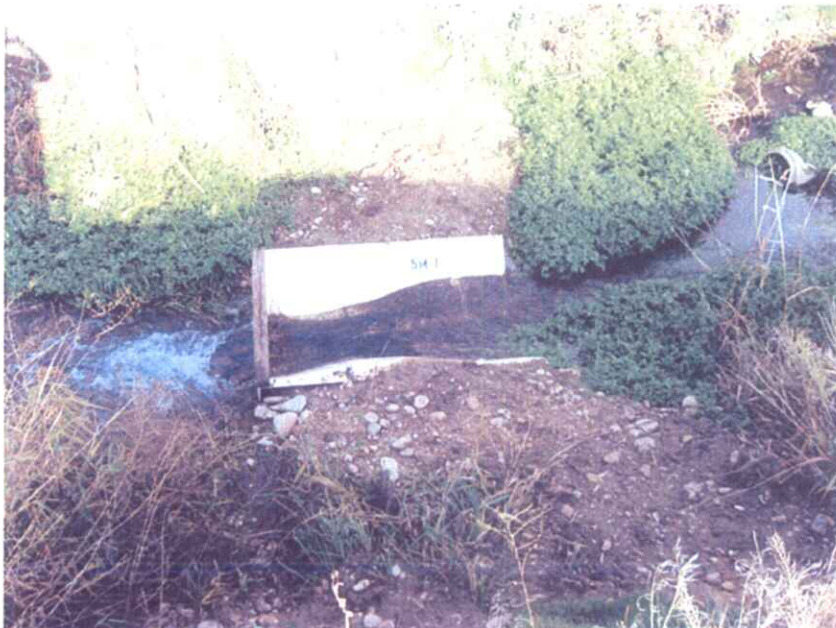
Photograph 2: Trapezoidal flume appears to be Plasti-Fab model 12" - 45° SRCRC.
