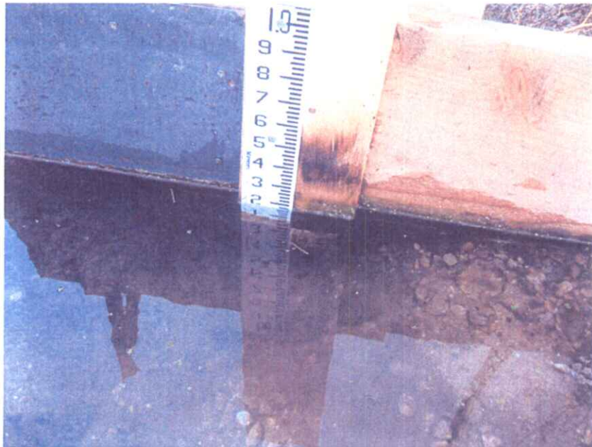
Photograph 5: Staff gage reading indicates 0.17 ft of head over Cipoletti Weir Crest. Approximate discharge at this stage is 2.2 cfs.
