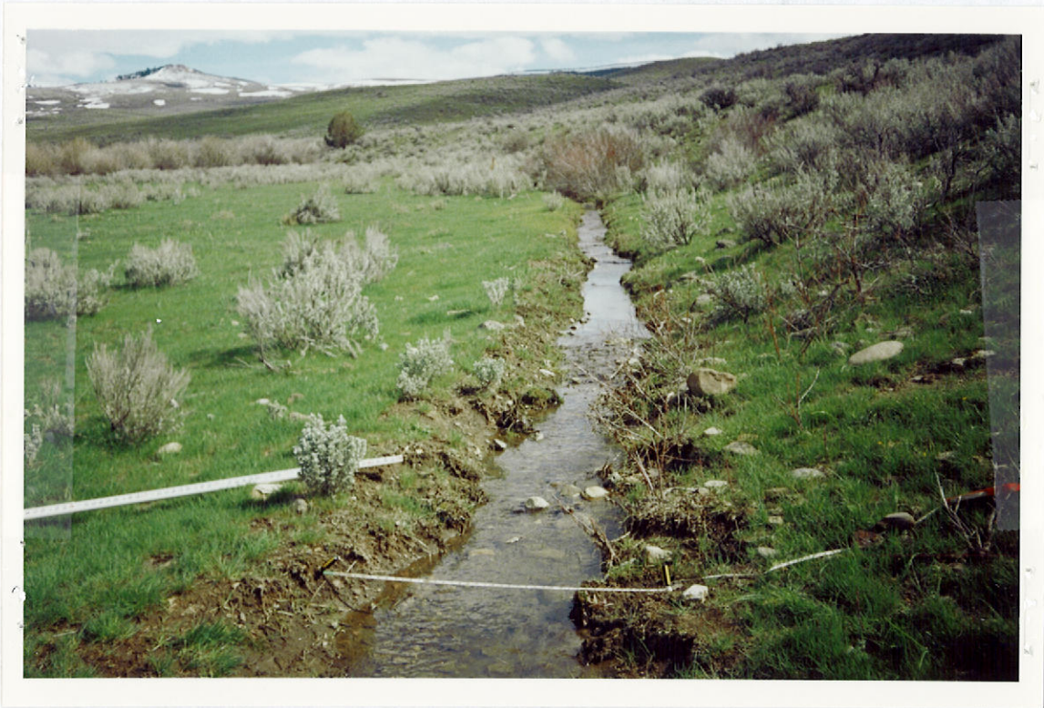
SOUTH DITCH. DOWNSTREAM CROSS SECTION. GOOD EXAMPLE OF DITCH, LOOKING UPSTREAM TOWARDS LEVEL.
