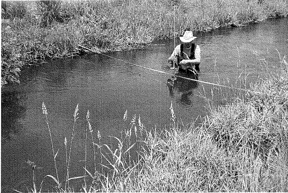
Photo 7. Measuring discharge in Johnson-Higby Ditch about 1.1 miles below headgate, above small private bridge.
