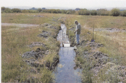
Portable flume in ditch flowing west.
