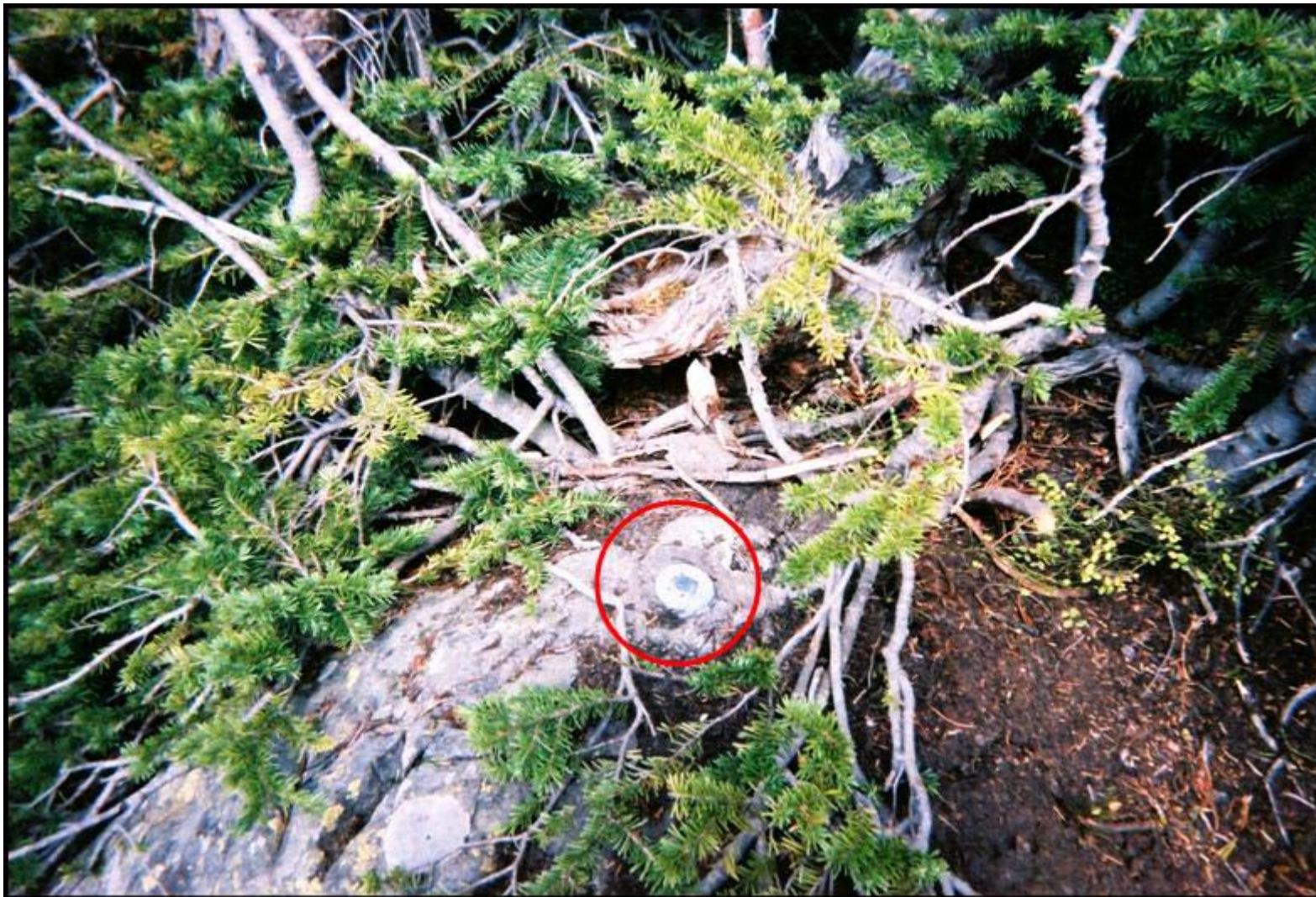
CP-1, Aluminum benchmark drilled and driven into rock, then covered with soil, rocks, and vegetation to hide the cap (inside circle).
