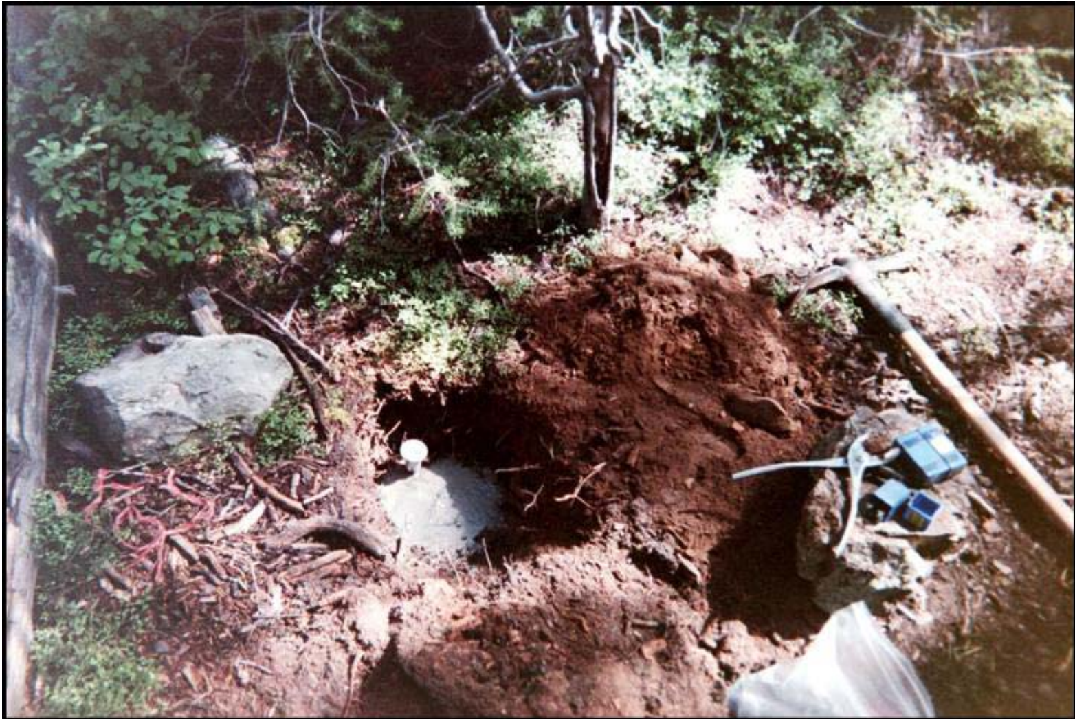
BM-1, The benchmark is a ½" re-bar set in concrete and capped with an aluminum cap. It is buried and hidden.
