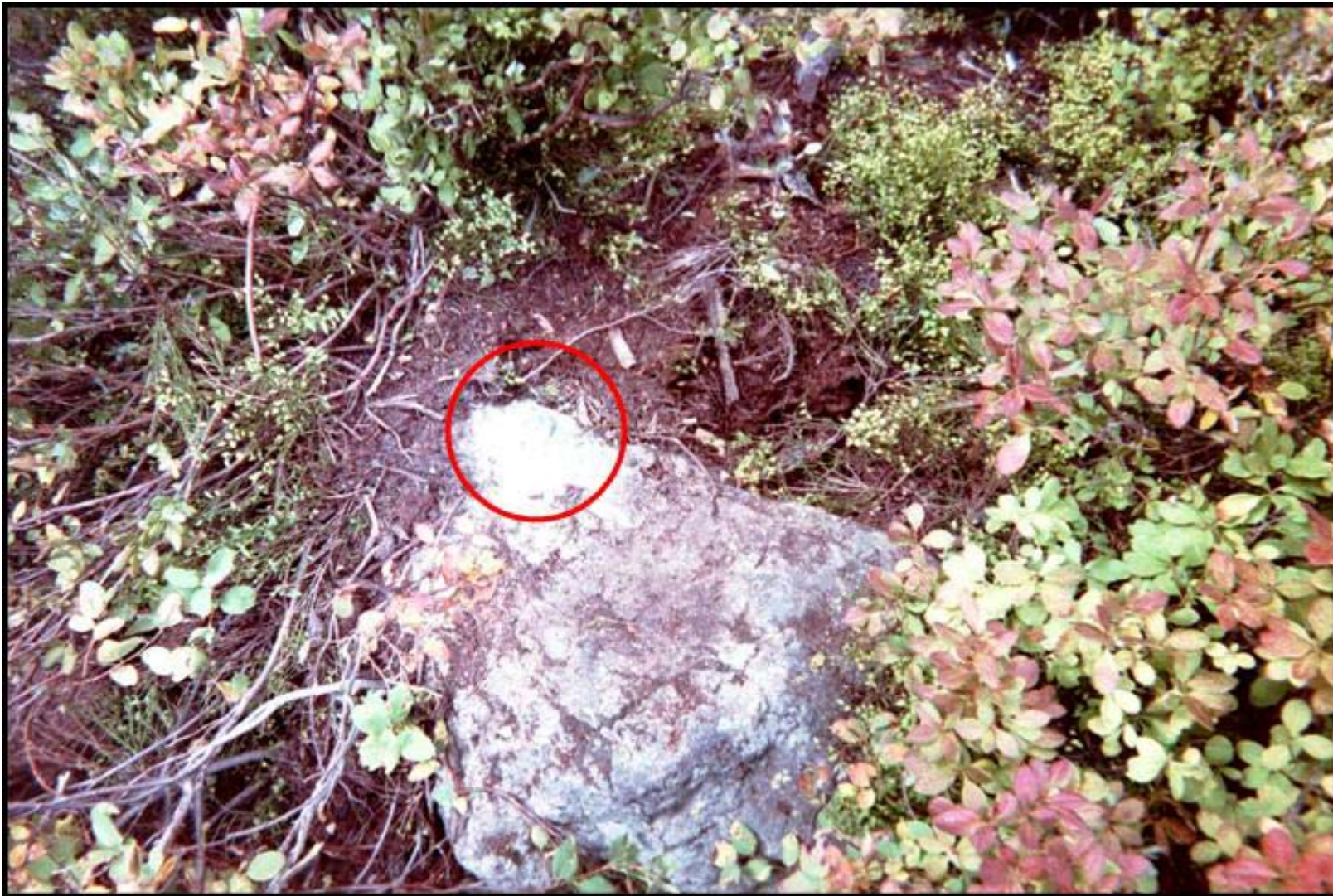
CP-1, Aluminum benchmark drilled and driven into rock, then covered with soil, rocks, and brush to hide the cap (inside circle).
