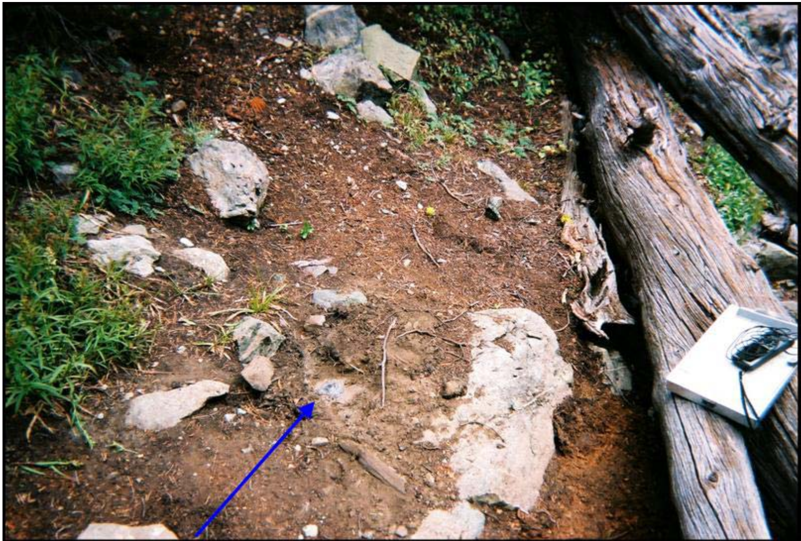
CP-1, Aluminum benchmark drilled and driven into rock, then covered with soil, and rocks, to hide the cap.
