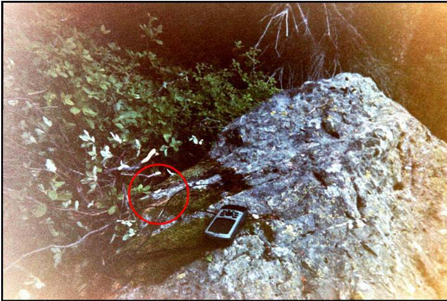
BM-1, Aluminum benchmark drilled and driven into rock, then covered with soil and rocks to hide the cap (inside circle).
