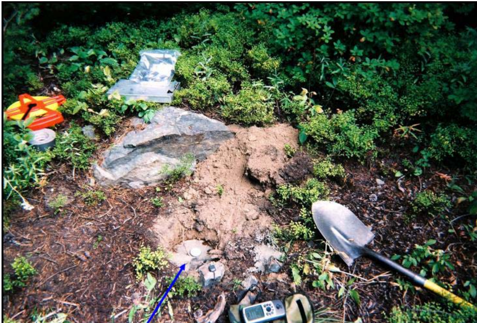
BM-1, rebar and aluminum cap incased in concrete and buried.
