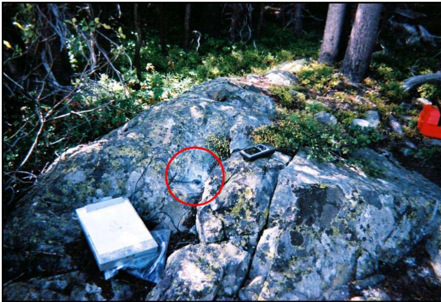
CP-1, Aluminum benchmark drilled and driven into rock, then covered with soil, and rocks, to hide the marker. Marker is located inside the circle.
