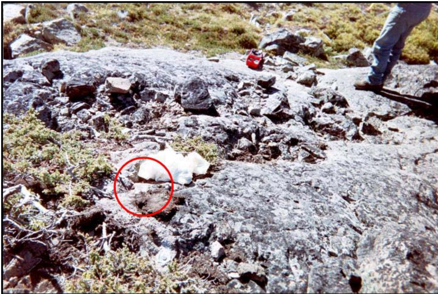
BM-1, Aluminum benchmark drilled and driven into rock, then covered with soil, rocks, and vegetation to hide the cap (inside circle).
