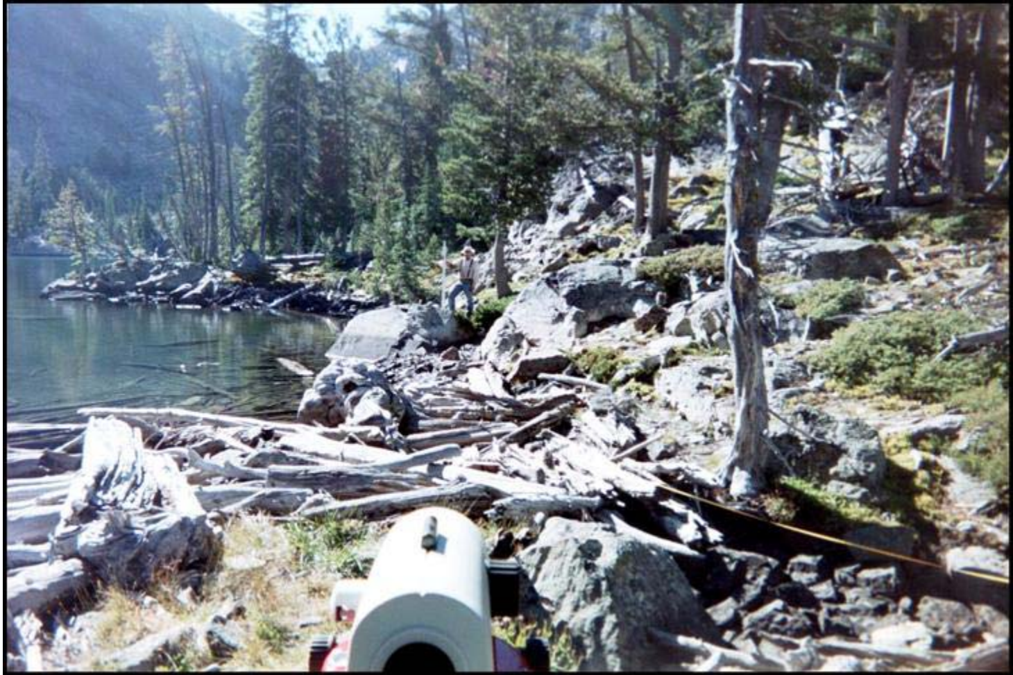
Shooting the aluminum benchmark CP-1 for elevation
