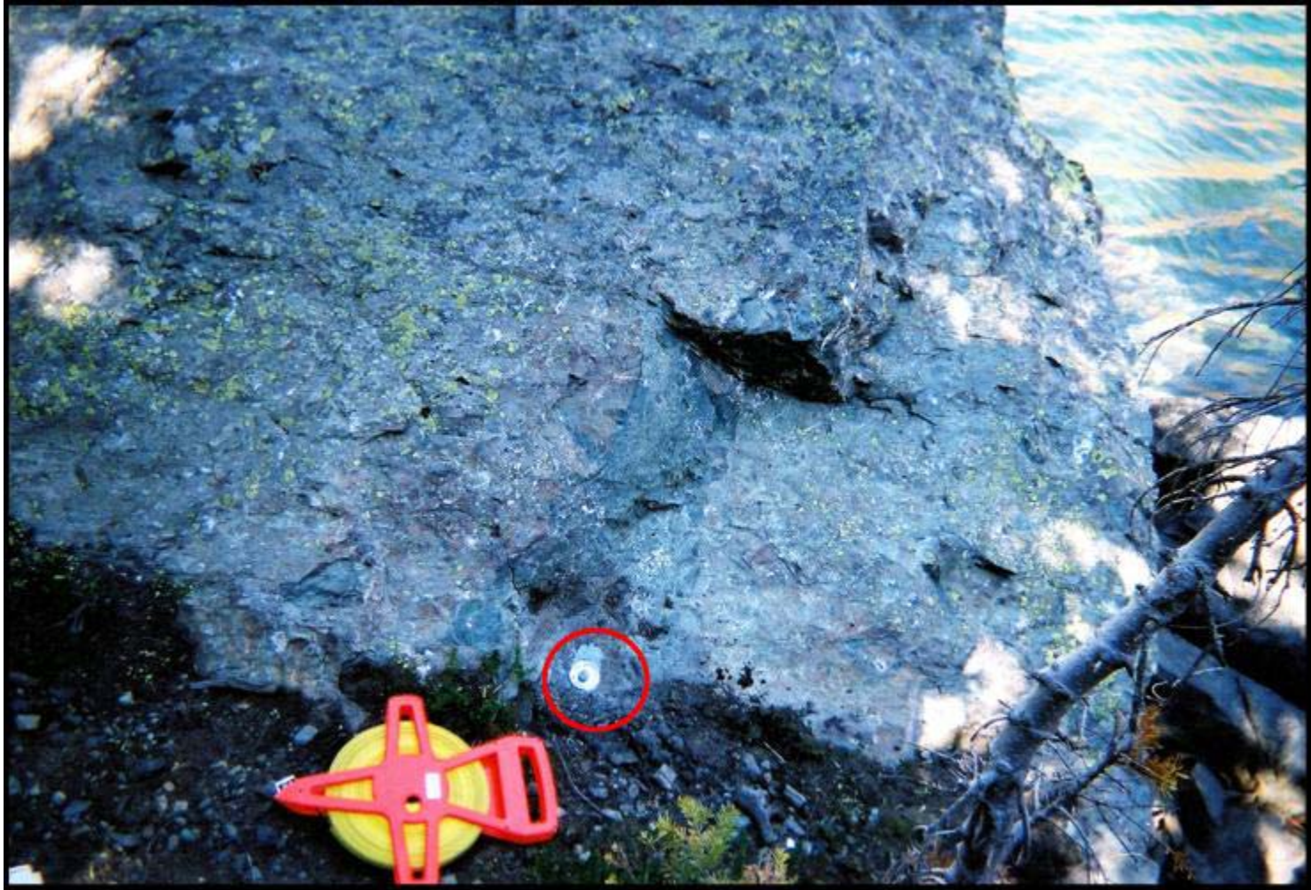
BM-1, An aluminum benchmark drilled and driven into the the rock and then covered with soil and rocks. BM-1 is inside the red circle.
