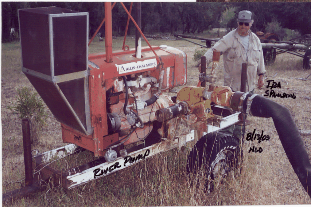
Photo 3. PORTABLE PUMP USED TO PUMP FROM SNAKE RIVER. RINS PORTABLE MINERLINE AND WHEEL-LINES —
